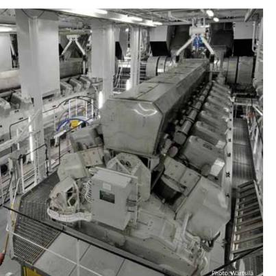
As the world's first manufacturer to use common rail electronic fuel injection on large, oil-fired diesel engines, Wärtsilä is one of the main innovators of embedded system development. Key to this innovation is Wärtsilä's engine control software. The main engine of the world's biggest cruising ship build by STX Finland: the Allures of the Seas.
